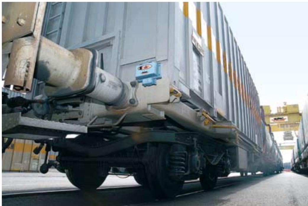
The system is based on innovative hardware components with GPS/GSM technology. A proactive information system matches the effective running data of every individual train with the selected timetable. "We receive high value qualitative information in real time without
