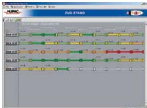
**E-train provides a visual representation of a train's status at predefined checkpoints.** Green means "on time", yellow means "up to 60 minutes late", red means "more than three hours late".
