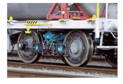
living near the tracks. During test and measurement runs with a Hupac wagon in summer 2006, the properties of the revolutionary bogie were checked and subsequently optimised. Leila's series maturity should be attained in autumn 2008, explained Josef-Meyer CEO Dominik Suter. The new device will only be successful "if railway companies and freight
