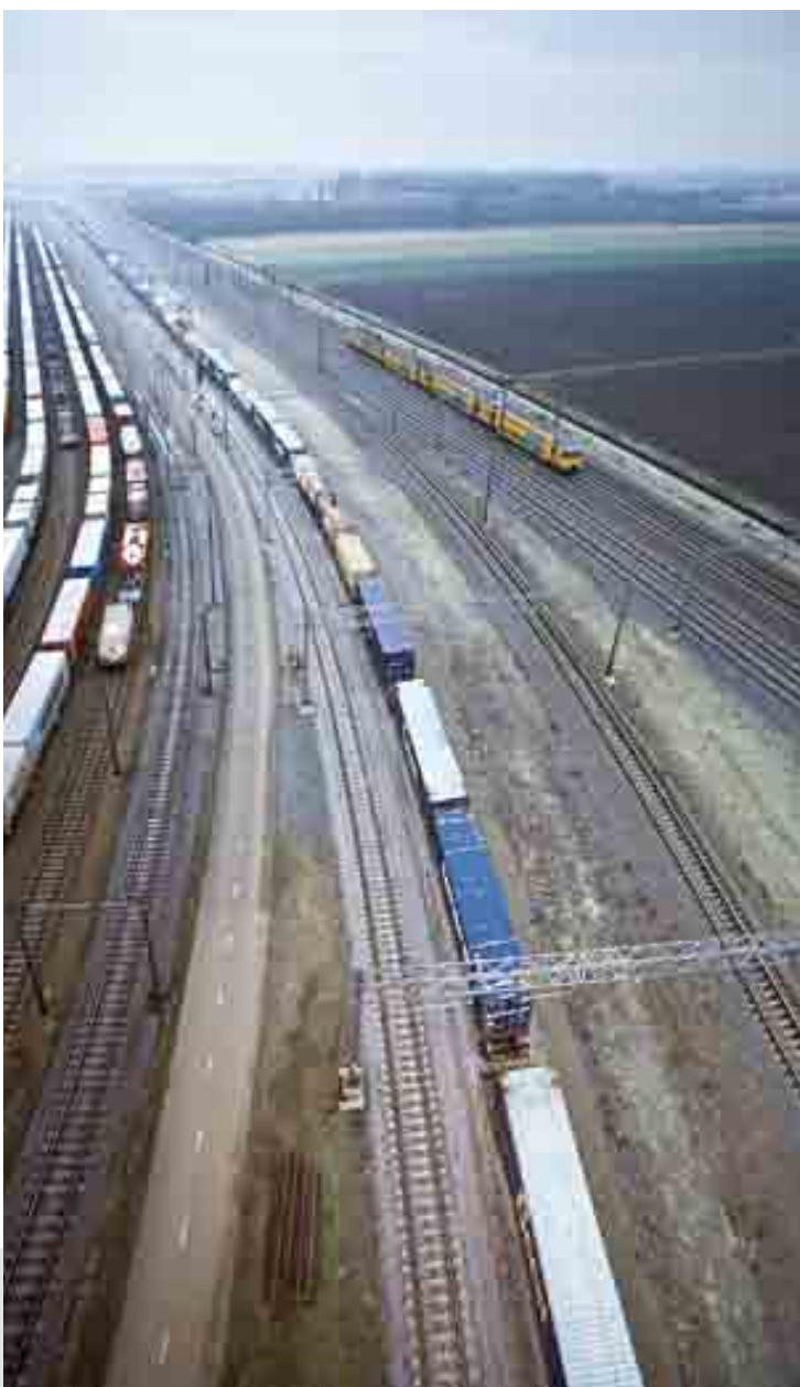
The 1,000 metre-long test composition by Deutsche Bahn carries thirty loaded Hupac wagons.
