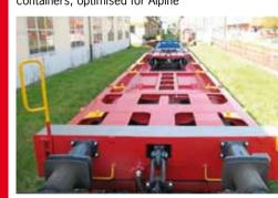
transit, in collaboration with the Ticino rolling stock manufacturer, Ferriere Cattaneo. Derived from the MEGA wagon, it features an increased load capacity and greater mileage. Environmental performance has also been improved: a combined synthetic pad and disc brake makes for lower noise levels. Testing of the prototype will run until the end of 2012.
