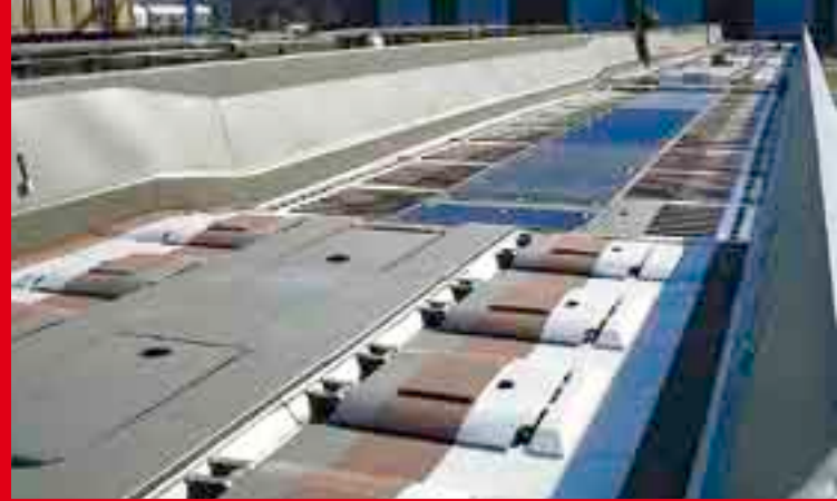
2004 - Extra-low-floor wagon for the Rolling Highway.
