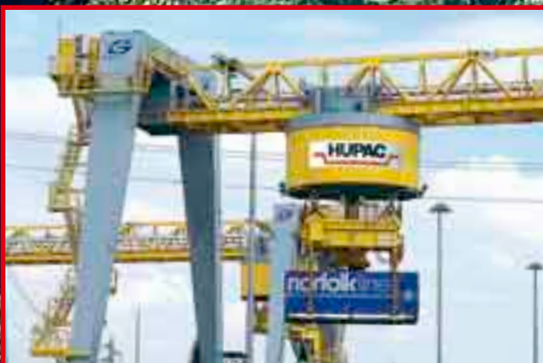
The powerful new generation of gantry cranes transfers the load units from the road to the tracks within minutes.
